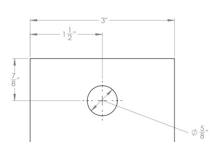
Note: To be installed on side of channel
